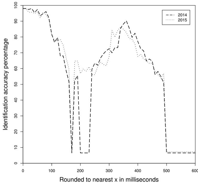
**Figure 2. Identification accuracy compared against rounding precision. All values in the data were rounded to a nearest millisecond value. The larger the millisecond value in the x-axis, the lesser the rounding precision. The y-axis expresses identification accuracy.**
